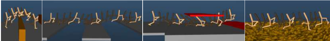
Figure 4: Walker skills : Time-lapse images of a representative Planar Walker policy traversing rubble; jumping over a hurdle; jumping over gaps and crouching to pass underneath a platform.
